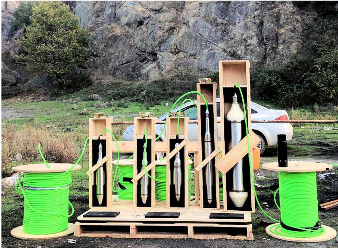
Part of the IESE Range of Sondes, including 1 Hz, 2 Hz and 4.5 Hz triaxial geophones
